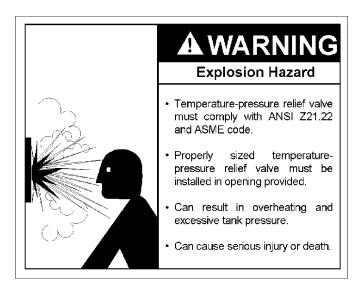
This heater is provided with a properly certified combination temperature - pressure relief valve by the manufacturer.
